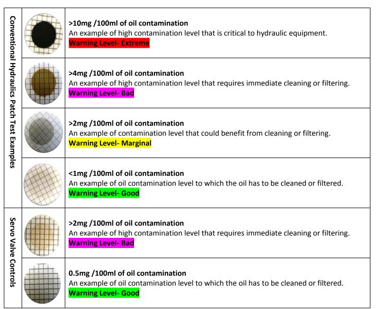
For reference, the grid lines in the membrane patches are approx. 100 $\mu$  wide
